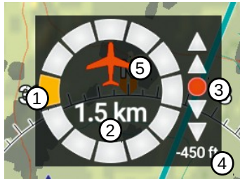
Figure 2.19: Threat classified as warning comes from left, distance is 1.5 km, about at the same visual level, 450 feet below.
