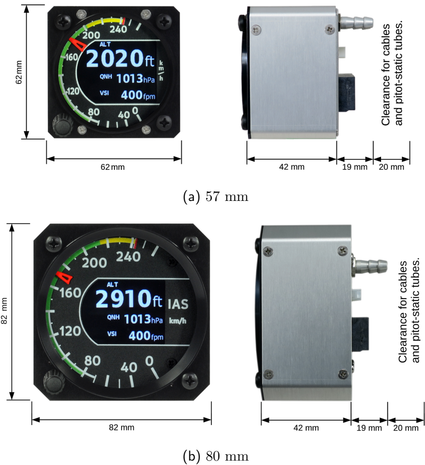
Figure 1: Front and side view with its principal dimensions.
