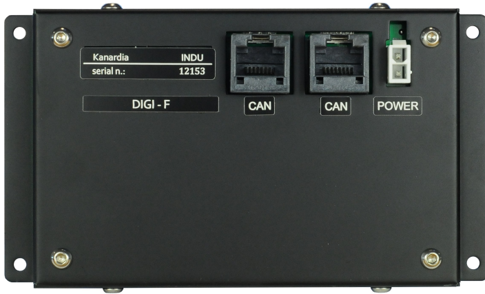
Figure 2: Back view of the Digi with connections.
