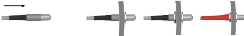
Figure 38: Inserting the OAT probe (left), cap is in place, tighten the internal nut, slide the insulation tube (right)
