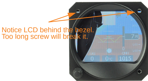
Figure 2: Example of broken LCD screen. Edge of the LCD display is visible behind the bezel.
