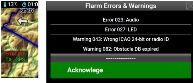
Figure 47: Left: a part of the main map screen, which shows the Flarm device status rectangle. Right: Flarm Error and Warning window. On top errors and warnings are displayed and the *Acknowledge* command at the bottom.
