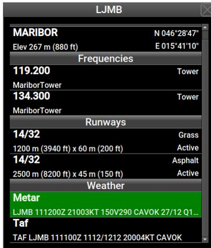
Figure 33: An example of the details window for LJMJB airfield.
