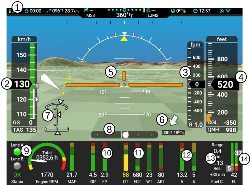
Figure 15: Illustration of the modern screen.
