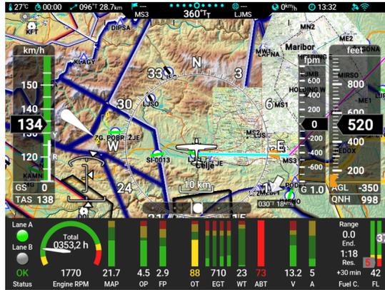
Figure 16: A moving map variant of modern screen.
