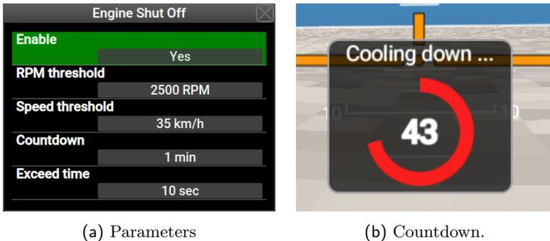
Figure 70: Engine shut down example.
