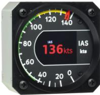
One or more slave round instruments can be added to the bus. They can show almost any value, which is available on the bus. The most typical are: air-speed indicator, altimeter, vertical speed indicator, engine RPM, rotor RPM, G-meter, etc. All indicators consists of a needle pointing to a scale and a LCD display. Pointer is driven by a stepper motor. Needle shows one value, but LCD display may show up to three different parameters.
