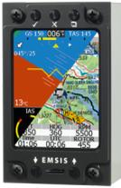
A small slave display (called EMSIS) comes in two forms. The first fits into 80 mm standard aviation opening, the second is larger with 3.5 inch diagonal and has more complex shape. They both can be viewed as small EFIS displays. EMSIS can show basic primary flight and engine monitor values.
