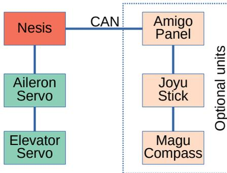
Figure 86: Main units of the autopilot system. Some units are optional.
