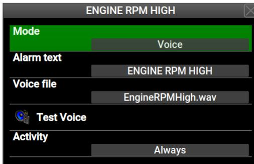
Figure 73: An example of alarm editor for the high engine RPM situation.
