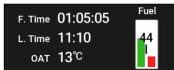
Figure 26: OAT, flight time, local time and fuel window.
