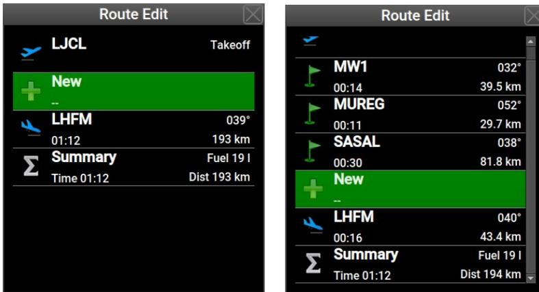
Figure 37: Route at the beginning, when only takeoff and landing airfields are known (left) and route at the end, when all intermediate points are entered (right).
