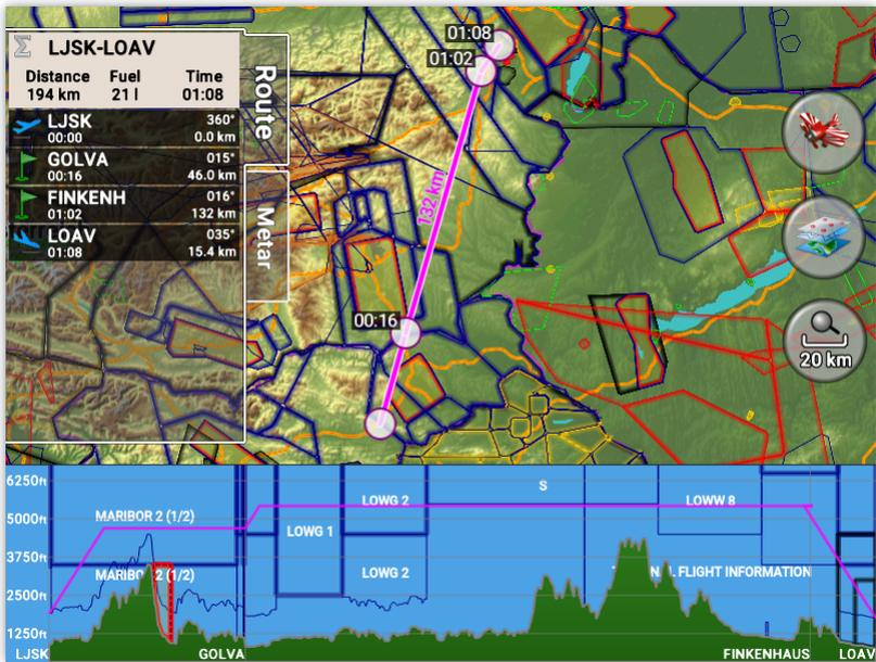
Figure 38: Example of route planning with touch screen.
