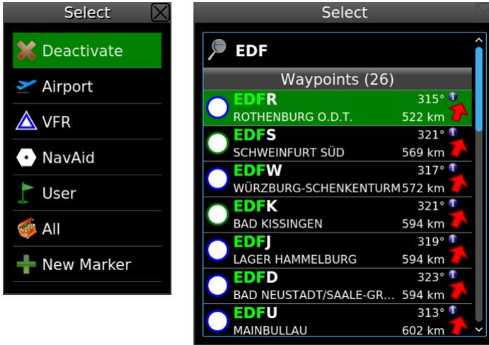
Figure 32: Waypoint options (left) and list of waypoints with active name filter (right).
