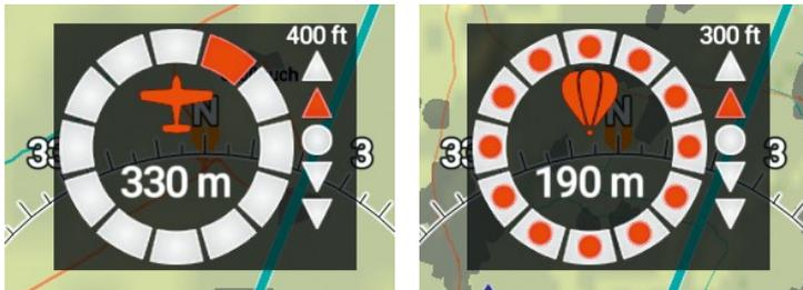
Figure 45: Left: Alert for an airplane, 330 meters away, slightly from right, 400 feet above and 10°- 30° above the horizon. Right: Alert for a balloon, 190 meters away, direction is not known, 300 feet above and 10°- 30° above the horizon.
