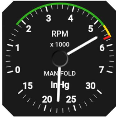
Figure 21: The combination of RPM and manifold pressure indicator.
