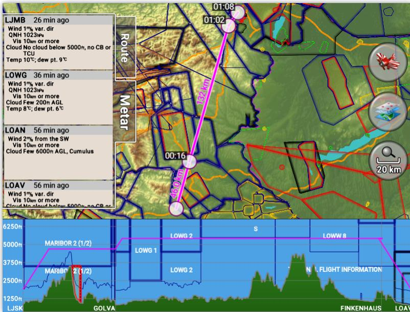
Figure 40: Example of METAR information along the route.
