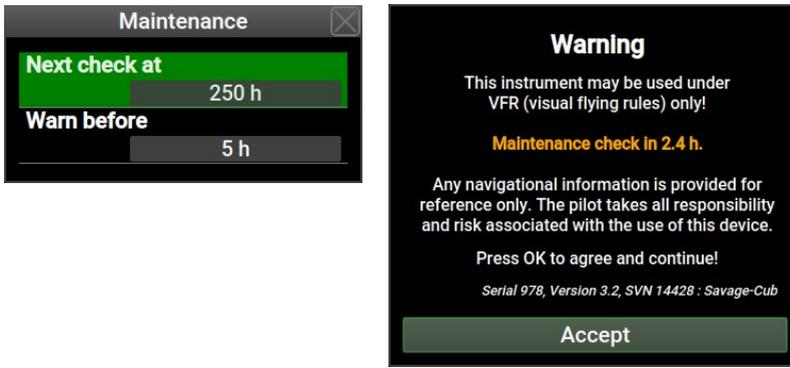
Figure 69: Left: Maintenance options. Right: Maintenance warning.
