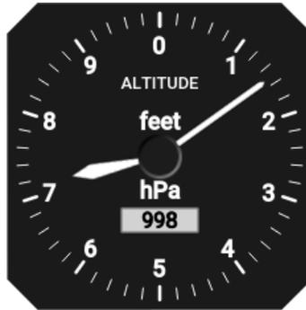
Figure 20: The altitude indicator with the scale given in feet.
