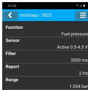
Figure 18: An example of fuel pressure sensor configuration.
