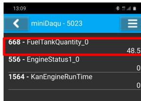
Figure 27: Checking tank indication value on the bus. Fuel level 1 is identified as FuelTankQuantity\_0. Value on the bus is always shown in liters.
