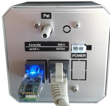
Figure 2: Blu inserted into an Indu device into one of the CAN ports.
