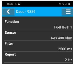
Figure 19: An example of fuel level sensor setting for channel E01.
